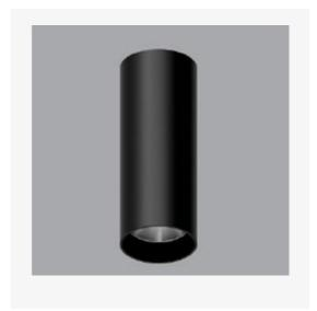
Artech Tenus surface architectural fixed LED downlight with ingress protection IP44. Total luminous flux up to 3000 lm with overall luminaire efficacy of 100 lm/W. Supplied with fixed output, DALI digital or phasecut dimmable driver, optional 3 -hour Basic or EMPRO emergency kit. Forged aluminum heat sink with die-cast white or black bezel.
