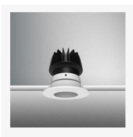
Artech Infra recessed architectural fixed LED downlight with ingress protection IP44. Total luminous flux up to 1408 Im with overall luminaire efficacy of 109Im/W. Supplied with fixed output, DALI digital or phase-cut dimmable driver, optional 3-hour Basic or EMPRO emergency kit. Forged aluminium heat sink with die-cast white or black bezel.
