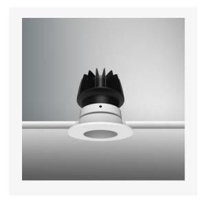
Artech Infra recessed architectural fixed LED downlight with ingress protection IP44. Total luminous flux up to 1408 lm with overall luminaire efficacy of 109lm/W. Supplied with fixed output, DALI digital or phase-cut dimmable driver, optional 3-hour Basic or EMPRO emergency kit. Forged aluminium heat sink with die-cast white or black bezel.
