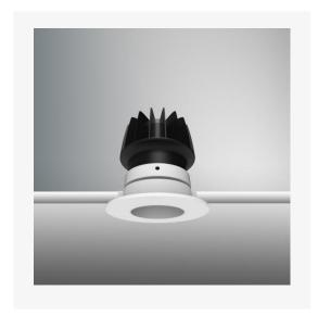
Artech Infra recessed architectural fixed LED downlight with ingress protection IP44. Total luminous flux up to 1408 Im with overall luminaire efficacy of 109Im/W. Supplied with fixed output, DALI digital or phase-cut dimmable driver, optional 3-hour Basic or EMPRO emergency kit. Forged aluminium heat sink with die-cast white or black bezel.
