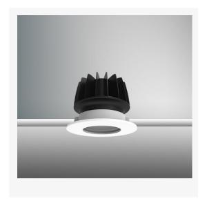
Artech Infra recessed architectural fixed LED downlight with ingress protection IP44. Total luminous flux up to 1408 Im with overall luminaire efficacy of 109Im/W. Supplied with fixed output, DALI digital or phase-cut dimmable driver, optional 3-hour Basic or EMPRO emergency kit. Forged aluminium heat sink with die-cast white or black bezel.
