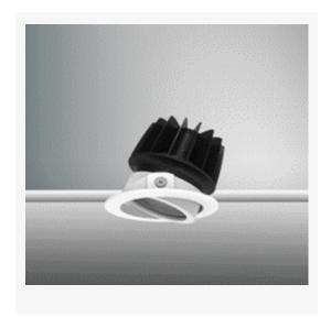
Artech Infra recessed architectural fixed LED downlight with ingress protection IP44. Total luminous flux up to 1408 Im with overall luminaire efficacy of 109lm/W. Supplied with fixed output, DALI digital or phase-cut dimmable driver, optional 3-hour Basic or EMPRO emergency kit. Forged aluminium heat sink with die-cast white or black bezel.
