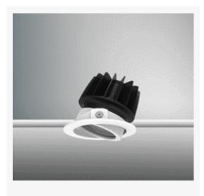
Artech Infra recessed architectural fixed LED downlight with ingress protection IP44. Total luminous flux up to 1408 lm with overall luminaire efficacy of 109lm/W. Supplied with fixed output, DALI digital or phase-cut dimmable driver, optional 3-hour Basic or EMPRO emergency kit. Forged aluminium heat sink with die-cast white or black bezel.
