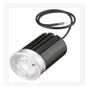
Artech Magna LED module, with high quality injection moulded TIR optic, COB LED, and extruded aluminium heatsink. Various lumen outputs, beam angles and colour temperatures available. 50mm diameter housing. High luminous efficacy up to 85 lm/W.
