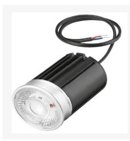
Artech Magna LED module, with high quality injection moulded TIR optic, COB LED, and extruded aluminium heatsink. Various lumen outputs, beam angles and colour temperatures available. 50mm diameter housing. High luminous efficacy up to 85 lm/W.
