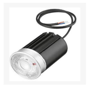
Artech Magna LED module, with high quality injection moulded TIR optic, COB LED, and extruded aluminium heatsink. Various lumen outputs, beam angles and colour temperatures available. 50mm diameter housing. High luminous efficacy up to 85 lm/W.
