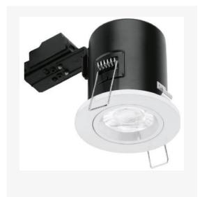
Artech Magna fire rated recessed IP65 LED luminaire with die-cast aluminium trim, steel housing, and pre-fitted GU10 LED lamp. Steel housing and intumescent material.
