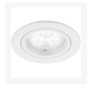
Artech Magna recessed shallow IP20 LED luminaire with die-cast aluminium trim, steel housing, and pre-fitted GU10 LED lamp. Steel housing and intumescent material.
