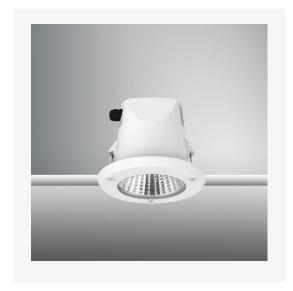
Artech Tenus recessed architectural fixed LED downlight with ingress protection IP65. Total luminous flux up to 1387lm with overall luminaire efficacy of 108 lm/W. Supplied with fixed output, DALI digital or phase-cut dimmable driver, optional 3 -hour Basic or EMPRO emergency kit. Forged aluminium heat sink with die-cast white or black colour finish.
