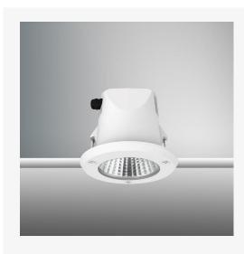
Artech Tenus recessed architectural fixed LED downlight with ingress protection IP65. Total luminous flux up to 1387lm with overall luminaire efficacy of 108 lm/W. Supplied with fixed output, DALI digital or phase-cut dimmable driver, optional 3 -hour Basic or EMPRO emergency kit. Forged aluminium heat sink with die-cast white or black colour finish.
