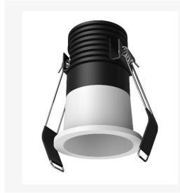
Artech Tenus recessed architectural fixed LED downlight with ingress protection IP20. Total luminous flux up to 260 Im with overall luminaire efficacy of 87 Im/W. Supplied with fixed output, DALI digital or phase-cut dimmable driver, due to dimensions of the Tenus Mini Range remote access driver required. optional 3 -hour Basic or EMPRO emergency kit. Forged aluminium heat sink with die-cast white or black bezel.
