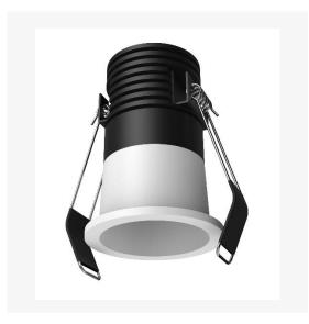
Artech Tenus recessed architectural fixed LED downlight with ingress protection IP20. Total luminous flux up to 260 lm with overall luminaire efficacy of 87 lm/W. Supplied with fixed output, DALI digital or phase-cut dimmable driver, due to dimensions of the Tenus Mini Range remote access driver required. optional 3 -hour Basic or EMPRO emergency kit. Forged aluminium heat sink with die-cast white or black bezel.
