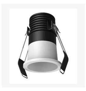
Artech Tenus recessed architectural fixed LED downlight with ingress protection IP20. Total luminous flux up to 560 lm with overall luminaire efficacy of 87 lm/W. Supplied with fixed output, DALI digital or phase-cut dimmable driver, due to dimensions of the Tenus Mini Range remote access driver required. optional 3 -hour Basic or EMPRO emergency kit. Forged aluminium heat sink with die-cast white or black bezel.
