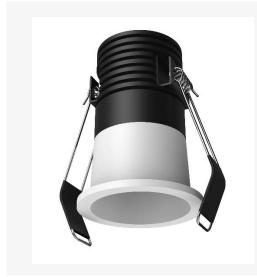
Artech Tenus recessed architectural fixed LED downlight with ingress protection IP20. Total luminous flux up to 560 Im with overall luminaire efficacy of 87 Im/W. Supplied with fixed output, DALI digital or phase-cut dimmable driver, due to dimensions of the Tenus Mini Range remote access driver required. optional 3 -hour Basic or EMPRO emergency kit. Forged aluminium heat sink with die-cast white or black bezel.
