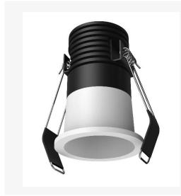
Artech Tenus recessed architectural fixed LED downlight with ingress protection IP20. Total luminous flux up to 560 Im with overall luminaire efficacy of 87 Im/W. Supplied with fixed output, DALI digital or phase-cut dimmable driver, due to dimensions of the Tenus Mini Range remote access driver required. optional 3 -hour Basic or EMPRO emergency kit. Forged aluminium heat sink with die-cast white or black bezel.
