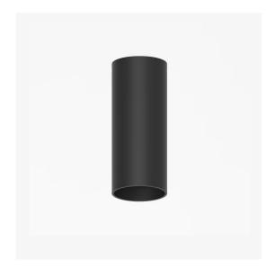
Artech Tenus surface architectural fixed LED downlight with ingress protection IP44. Total luminous flux up to 3000 lm with overall luminaire efficacy of 100 lm/W. Supplied with fixed output, DALI digital or phase-cut dimmable driver, optional 3 -hour Basic or EMPRO emergency kit. Forged aluminium heat sink with die-cast white or black bezel.
