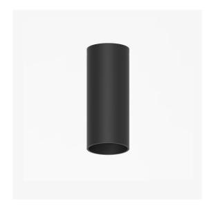
Artech Tenus surface architectural fixed LED downlight with ingress protection IP44. Total luminous flux up to 3000 lm with overall luminaire efficacy of 100 lm/W. Supplied with fixed output, DALI digital or phase-cut dimmable driver, optional 3 -hour Basic or EMPRO emergency kit. Forged aluminium heat sink with die-cast white or black bezel.
