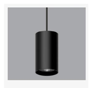
Artech Tenus pendant architectural fixed LED downlight with ingress protection IP44. Total luminous flux up to 3000 Im with overall luminaire efficacy of 100 Im/W. Supplied with fixed output, DALI digital or phase-cut dimmable driver, optional 3 -hour Basic or EMPRO emergency kit. Forged aluminium heat sink with die-cast white or black bezel.
