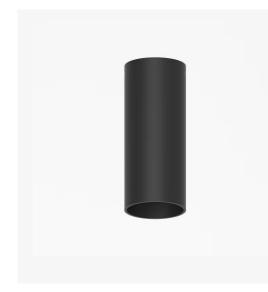
Artech Tenus surface architectural fixed LED downlight with ingress protection IP44. Total luminous flux up to 3000 lm with overall luminaire efficacy of 100 lm/W. Supplied with fixed output, DALI digital or phase-cut dimmable driver, optional 3 -hour Basic or EMPRO emergency kit. Forged aluminium heat sink with die-cast white or black bezel.
