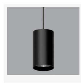
Artech Tenus pendant architectural fixed LED downlight with ingress protection IP44. Total luminous flux up to 3000 lm with overall luminaire efficacy of 100 lm/W. Supplied with fixed output, DALI digital or phase-cut dimmable driver, optional 3 -hour Basic or EMPRO emergency kit. Forged aluminium heat sink with die-cast white or black bezel.
