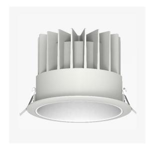
Artech Tenus recessed architectural fixed LED downlight with ingress protection IP44. Total luminous flux up to 2425 lm with overall luminaire efficacy of 125 lm/W. Supplied with fixed output, DALI digital or phase-cut dimmable driver, optional 3 -hour Basic or EMPRO emergency kit. Forged aluminium heat sink with die-cast white or black bezel.
