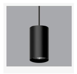
Artech Tenus pendant architectural fixed LED downlight with ingress protection IP44. Total luminous flux up to 3000 lm with overall luminaire efficacy of 100 lm/W. Supplied with fixed output, DALI digital or phase-cut dimmable driver, optional 3 -hour Basic or EMPRO emergency kit. Forged aluminium heat sink with die-cast white or black bezel.
