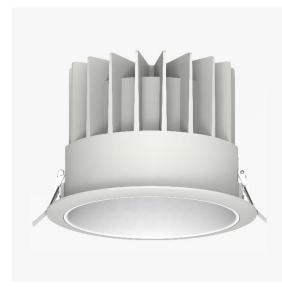
Artech Tenus recessed architectural fixed LED downlight with ingress protection IP44. Total luminous flux up to 2425 lm with overall luminaire efficacy of 125 lm/W. Supplied with fixed output, DALI digital or phase-cut dimmable driver, optional 3 -hour Basic or EMPRO emergency kit. Forged aluminium heat sink with die-cast white or black bezel.
