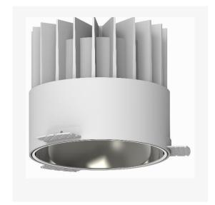
Artech Tenus recessed architectural fixed LED downlight with ingress protection IP44. Total luminous flux up to 2425 lm with overall luminaire efficacy of 125 lm/W. Supplied with fixed output, DALI digital or phase-cut dimmable driver, optional 3 -hour Basic or EMPRO emergency kit. Forged aluminium heat sink with die-cast white or black bezel.
