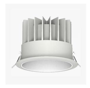
Artech Tenus recessed architectural fixed LED downlight with ingress protection IP44. Total luminous flux up to 3360 lm with overall luminaire efficacy of 125 lm/W. Supplied with fixed output, DALI digital or phase-cut dimmable driver, optional 3 -hour Basic or EMPRO emergency kit. Forged aluminium heat sink with die-cast white or black bezel.
