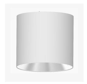
Artech Tenus surface architectural fixed LED downlight with ingress protection IP44. Total luminous flux up to 5000 Im with overall luminaire efficacy of 125 Im/W. Supplied with fixed output, DALI digital or phase-cut dimmable driver, optional 3 -hour Basic or EMPRO emergency kit. Forged aluminium heat sink with die-cast white or black bezel.
