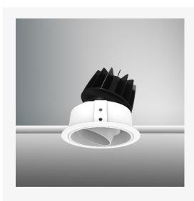
Artech Tenus recessed architectural fixed LED downlight with ingress protection IP44. Total luminous flux up to 1408 lm with overall luminaire efficacy of 109 lm/W. Supplied with fixed output, DALI digital or phase-cut dimmable driver, optional 3 -hour Basic or EMPRO emergency kit. Forged aluminium heat sink with die-cast white or black bezel.
