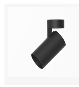
Tenus 90 is an elegant directional surface spotlight, with high quality aluminium housing and discrete hinge design allowing for concise adjustment. Total luminous flux up to 3000 Im with overall luminaire efficacy of 100 Im/W. Supplied with fixed output, DALI digital or phase-cut dimmable driver, optional 3 -hour Basic or EMPRO emergency kit. Forged aluminium heat sink with diecast white or black bezel.
