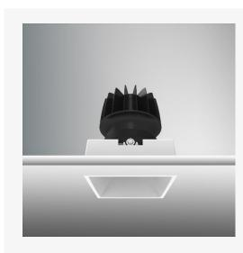
Artech Tenus recessed architectural fixed LED downlight with ingress protection IP44. Total luminous flux up to 1408 Im with overall luminaire efficacy of 109 Im/W. Supplied with fixed output, DALI digital or phase-cut dimmable driver, optional 3 -hour Basic or EMPRO emergency kit. Forged aluminium heat sink with die-cast white or black bezel.
