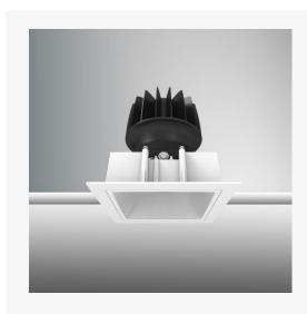
Artech Tenus recessed architectural fixed LED downlight with ingress protection IP44. Total luminous flux up to 1900 lm with overall luminaire efficacy of 109 lm/W. Supplied with fixed output, DALI digital or phase-cut dimmable driver, optional 3 -hour Basic or EMPRO emergency kit. Forged aluminium heat sink with die-cast white or black bezel.
