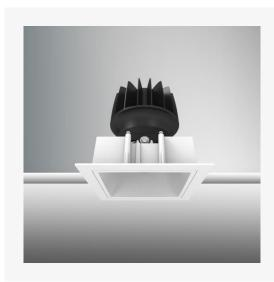
Artech Tenus recessed architectural fixed LED downlight with ingress protection IP44. Total luminous flux up to 1900 lm with overall luminaire efficacy of 109 lm/W. Supplied with fixed output, DALI digital or phase-cut dimmable driver, optional 3 -hour Basic or EMPRO emergency kit. Forged aluminium heat sink with die-cast white or black bezel.
