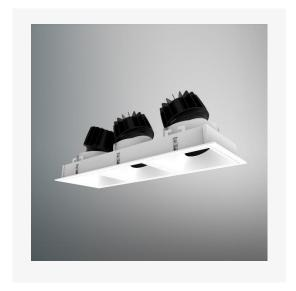
Artech Tenus recessed architectural fixed LED downlight with ingress protection IP44. Total luminous flux up to 724 lm with overall luminaire efficacy of 109 lm/W. Supplied with fixed output, DALI digital or phase-cut dimmable driver, optional 3 -hour Basic or EMPRO emergency kit. Forged aluminium heat sink with die-cast white or black bezel.
