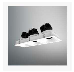
Artech Tenus recessed architectural fixed LED downlight with ingress protection IP44. Total luminous flux up to 1006 lm with overall luminaire efficacy of 109 lm/W. Supplied with fixed output, DALI digital or phase-cut dimmable driver, optional 3 -hour Basic or EMPRO emergency kit. Forged aluminium heat sink with die-cast white or black bezel.
