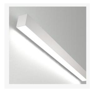
Architectural linear LED system for Wall mounted applications. Total luminous flux of up to 3098 lm with overall luminaire efficacy 130 lm/W. Supplied with fixed output or DALI digital dimmable drive. Optional basic 3hr, self-test or EMPRO emergency kit providing a total of 520lm in emergency mode. Aluminium extruded body in white, black, or silver finish. MPO (UGR 19) optic with high lumen output and luminance intensity control.
